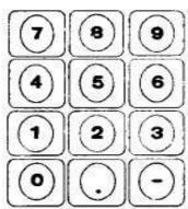
**15 The NUMERIC KEYBOARD** uses the ten-key entry system with provision for entry of a decimal point and a negative sign. Keyboard entries are automatically stored in the M register.
