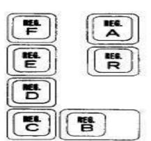
**18 The REGISTER ADDRESS KEYS A, B, C, D, E, F and R** identify the corresponding registers. The operating register M has no keyboard identification since the computer automatically relates all instructions to the M register unless instructed otherwise.
